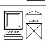
5. To install the post cap, set it in place on top of the post and strike with a rubber mallet to drive the post cap onto the post. Silicone or water based caulking may be used to secure the post cap and base trim.
