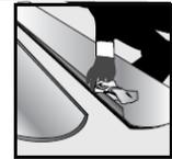
3. Apply FRP Adhesive to all connecting surfaces on both halves. FRP Adhesive can be used between 50°F (10°C) and 90°F (32°C). Cure time increases with lower temperatures.
