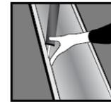
4. Align the halves around the structural support and bring completely together. Secure using straps along the length of the column and pull tight.
