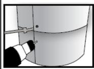
5. After adhesive is cured, remove the zip-ties. Remove any excess adhesive by cutting, scraping, or sanding with a dustless sander.
