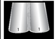
2. Pro-Fusion split columns are designed with a convenient full length lap to aid in reassembly of the column. For highest bond strength, wipe down lap and mating surfaces with acetone or naphtha to ensure complete removal of debris.
