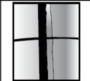
4. Join the two column halves together by tightening the zip-ties and replace the screws into the pre-drilled holes. Using a power or hand screw driver, tighten the screws only enough to align the two halves to produce a smooth finish.
