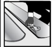
3. Stand column halves in position around the beam or structure that the column will wrap. Loosely fit the zip-ties from the split kit around the column to hold the halves together. Allow enough space to liberally apply FRP adhesive to all connection surfaces on both halves. FRP adhesive can be used between 50°F (10°C) and 90°F (32°C). Cure time increases with lower temperatures.
