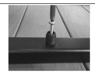
3. Cut 10" Support Block (F) to required length and press over the Support Block Connector installed in step 2. Support block is typically cut at 2", but can be cut longer based on your project needs.
