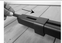
6. Place Bottom Rail (B) between posts ensuring rail is level and support block is properly installed and grooved side of rail is facing upward. Place provided 2" Foam Blocks Spacers (N) under each end of the Bottom Rail to help level it and aid in the installation. Slide Bottom Brackets (E) firmly against and centered on the post and secure with 2ea, required #10 x 1" self drilling screws (H).
