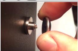
locknut as close as possible using a cut-off wheel or hacksaw. Press the nut cap over the locknut. Press the cap onto the fitting.
