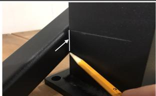
7. Place the Top Rail (A) with the bottom side of the rail facing up next to the Bottom Rail (B), and duplicate the marks from the bottom rail cut line onto the top rail. Now mark the top rail 5/8" shorter on each end; this is the cut line for top rail.
