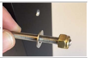
3. Slide line fittings with required round black washers onto the cables while twisting in a clockwise motion until the fittings are fully seated in the end post. Pull the bare ends to remove as much slack as possible.
