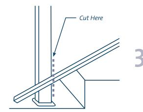
Place the top stair rail directly over the bottom rail while making sure that the holes are aligned. Tape them together temporarily so they will not move during the angle marking. Lay the rails on the stairs against the post. Make sure the holes in the rails are evenly distributed between the posts before marking the angle to be cut on both rails with a pencil.
