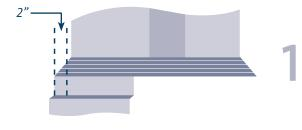
Draw a line with a pencil at 2" from the edge of your deck or balcony (perimeter line) to guide your installation. Start your installation from a corner bottom of the stair.
