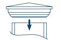
Finish by placing the top cap on each post. Use PVC glue or silicone caulking to attach the caps.
