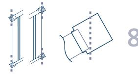
The brackets for the stair railing section are extended to accommodate cutting the back side (side to be mounted on the post) at the angle required for the steps, "stair-angle".
