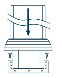
Install the first post by attaching the ACQ pad and internal reinforcement post to the bottom surface. Slide the post sleeve over the internal reinforcement post and attach the post sleeve to the ACQ pad. Finish by sliding the post base trim to the bottom of the post to cover the post base.
