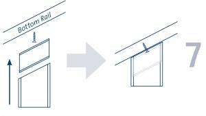
Screw the stair support components (prepared in Step 4) to the underside of the bottom rail.
