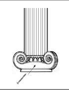
3. Place the assembled column on its side, then slide the base on the column shaft. Ensure the base aligns with the capital (do not secure).
