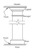
4. To assemble and install the capital and base, drill and counter-sink through flat surface of both halves of the base with 1/8" bit. Install both halves to the bottom of the column, flush with the floor, and secure them with the provided screws on all sides. Repeat this process with the capital at the top of the column. If needed, caulk between seams for a finished look.
